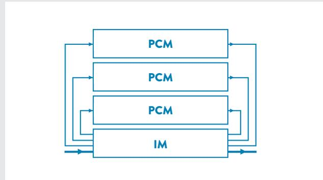
**PCM:** The power converter module is available in a 25kV, 31kVA and 37kVA configuration. These PCMs can be paralleled up to at least 20 units (5 per system).
